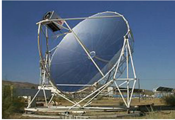
Fig. 16.5 Photograph of a Stirling solar engine
